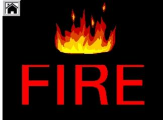
By code, the fire system and the fans must be interconnected. It most jurisdictions the sequence of operation requires the exhaust fan to remain on or turn on while the supply fan must turn off or remain off. The programming of the Smart Hood system will accomplish this sequence. Once the fire system is reset you will see either one of these screens.
