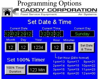
**Changing the 100% Timer duration:** Hit the "Setup" button. Hit the 100% Timer Duration button to bring up the user input box. The default time is 5 minutes and we recommend not exceeding 15 minutes.
