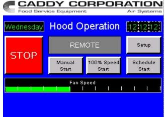
The "Remote" mode is used when the facility would like to take control of the schedule for when the hoods will turn on and off during the day. The terminal block in the VFD cabinet will have two terminals marked "Remote Start". When 120V is applied to those terminals the Smart Hood system will start the fans. During "Remote Start" mode the fans will still vary their speed based on temperature values.
