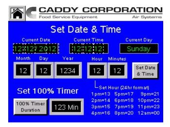
The first time you enter the program, you will be asked to set up the time and date. You can modify the month by pressing inside the month field with the heavy gray border. Continue doing this for each field. The clock must be set using the 24 hour format. For your convenience, we have provided a chart in the lower right hand corner. Once each field is accurate, you must press the "Set Date & Time" button on the right side of the screen to update the settings.
